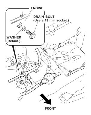
12. Install the new aluminum washer and the engine block heater to the bolt hole using a 24 mm socket and torque wrench. Torque the engine block heater to 60 N·m (44 lbf·ft).
