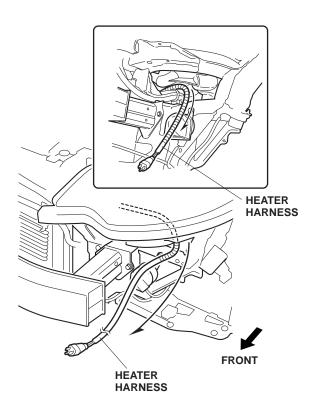
18. Secure the fifth wire tie with clip, which you installed on the heater harness, to the vehicle frame.
